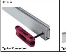
Most horizontal extrusion connections have a patented expandable lock. This lock inserts into the groove of an opposing extrusion. Tightening the lock with the Hex Key Tool expands the lock and creates a strong positive connection.
