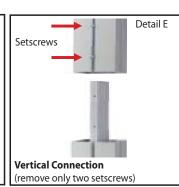
When vertical extrusions are packed in portable cases rather than crates or tubs, they must be broken down into smaller section which then require assembly.
